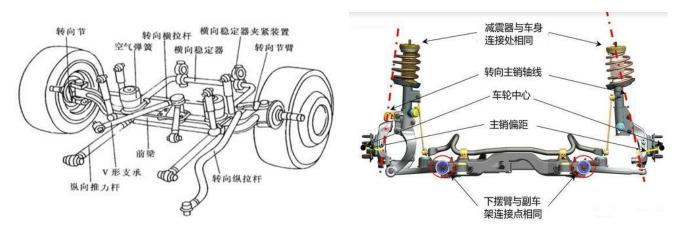
If the car tie rod is straight, you can loosen the locking bolt of the joint at both ends of the tie rod first, and twist the tie rod with a pipe wrench to elongate or shorten the tie rod. When the tie rod elongates, the front bundle value increases, while the tie rod shortens, the front bundle value decreases. Tighten the bolts until the front bundle meets the standard.
